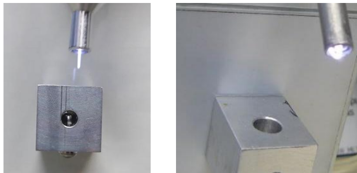
Fig. 3: Igniting the plasma using the starter box (left) and eventual arcing after ignition (right).
