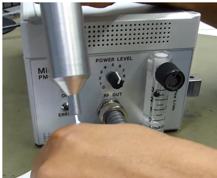
Fig. 1: Photo of the MiniJet-R with a cold plasma for general applications (no Photoshop, but overexposure of the plasma).
