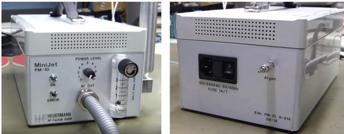
Fig. 1: Front and back views of the actual 10W generator with standard gas flow meter.
