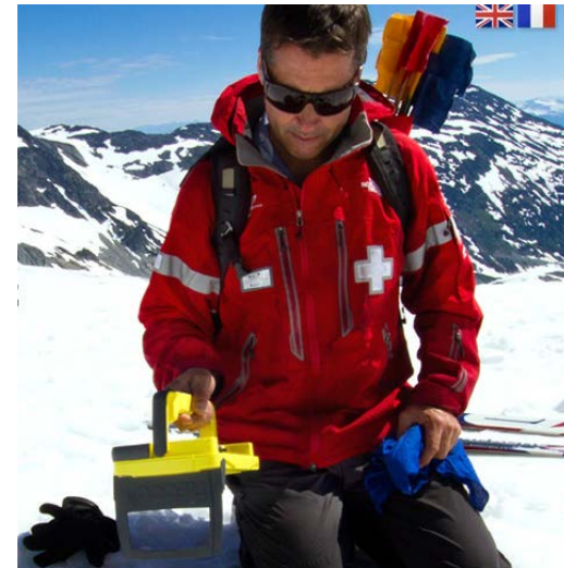
RECCO Interrogator, P_{TX} = 1.7 \text{ W CW @ 917 MHz} 5 El. Yagi 917 MHz, 4 Element Patch Array 1834 MHz
