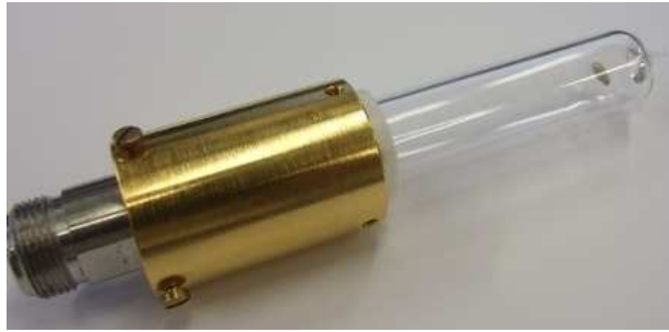
Bild 8.17: First demonstrator of an electrodeless low pressure discharge lamp operating at 2.45 GHz.
