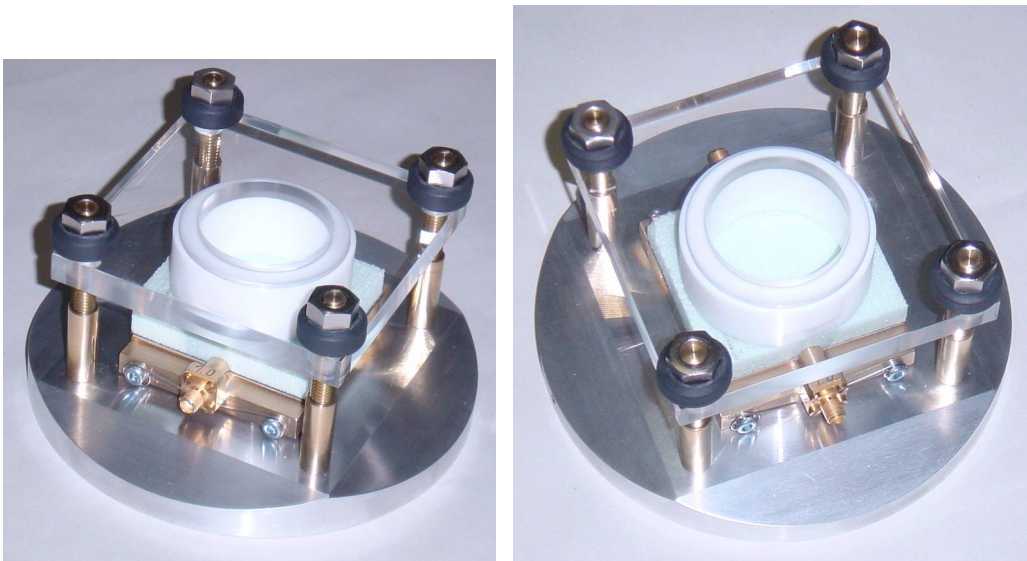
Fig. 1: Test fixture with base plate, SMA coupling elements and pressure block
