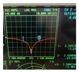
Case 2: Matching an open to 50  $\Omega$  (with a 1m cable)
