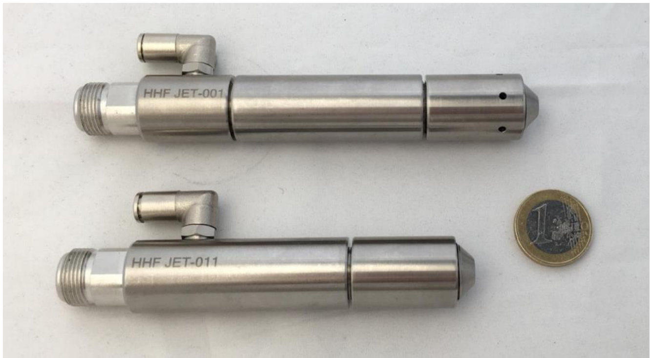
Abb. 1: PS-series plasma jets (top to bottom: PS and PS-Ar).
