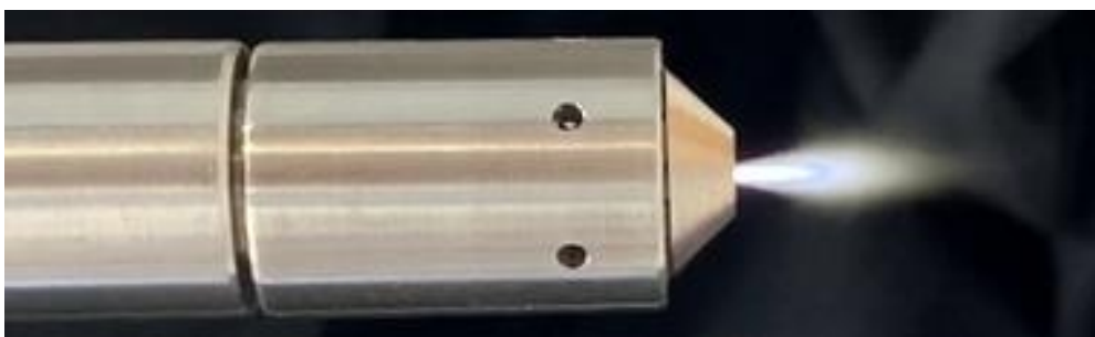
Fig. 3: PS plasma jet at 250 W for surface cleaning.
