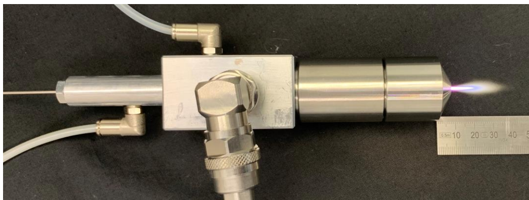
Fig. 1: The PC-SF3 jet at about 250 W with adaptor containing a stainless steel tube to separate gas 1 from eventual powder or aerosol to be treated.
