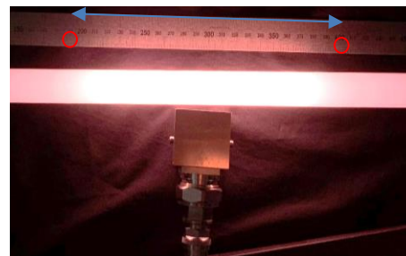
Fig. 3: Improving the operational matching by increasing the distance between coupler and applicator for 30 W at 2.46 GHz using a fluorescent lamp (on left -1 dB matching at < 1 mm, whereas ~ 3 mm brings up -4 dB matching to the right side).
