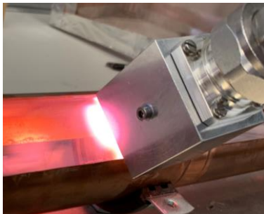
Fig. 1: Plasma produced with the CC1000 in a glass cylinder at 10 mbar with argon using 250 W.
