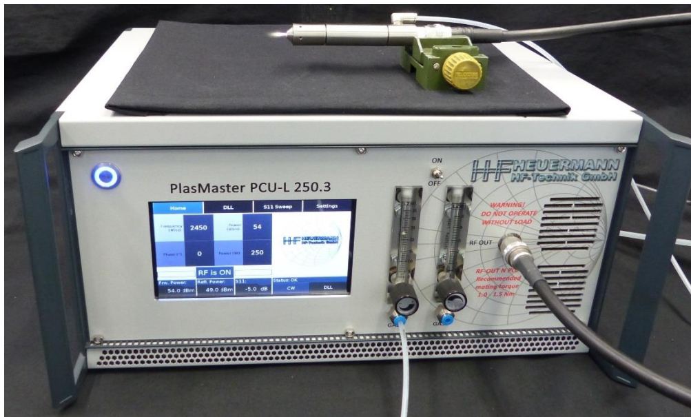
Fig. 1: The PlasMaster PCU-L 250.3 with a PS plasma jet.
